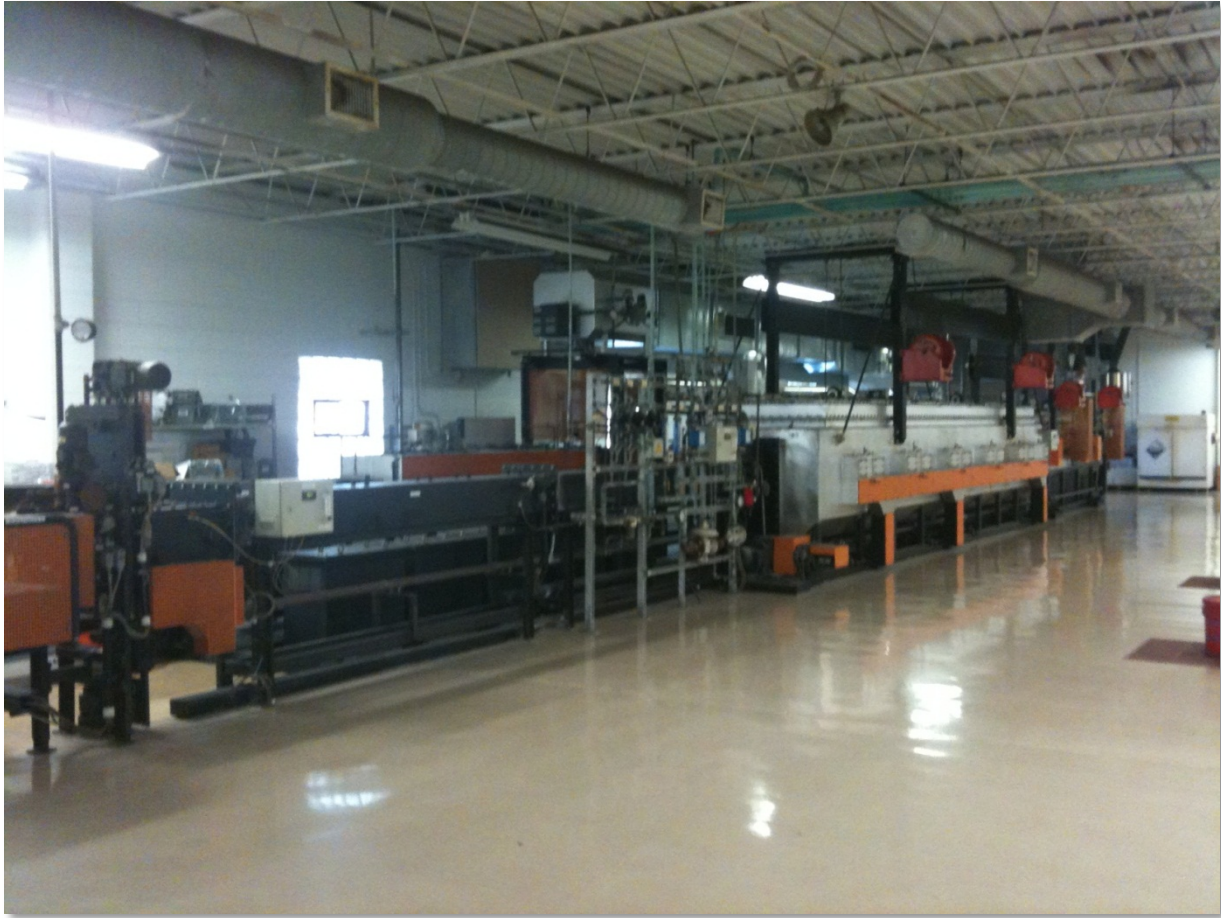
Smith Continuous Debind / Sintering Furnace
